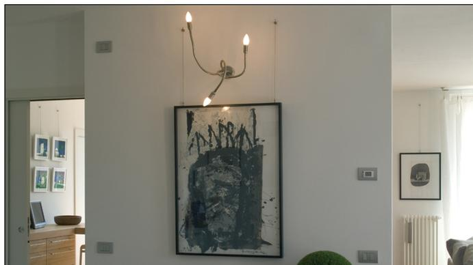
System for wall-mounted display of artworks, pictures, photographs, composed of an element fixed to the wall which supports a stainless steel cable: along the length of the cable it is possible to mount one or more accessories, with a hook or which make it possible to make a noose from which to hang the pictures. Ideal for displays on walls which otherwise present difficulties for fixing pictures such as sliding doors or plasterboard.
